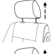
2. Simultaneously press and hold both the adjust/release button and the unlock/remove button, then pull up on the head restraint.
